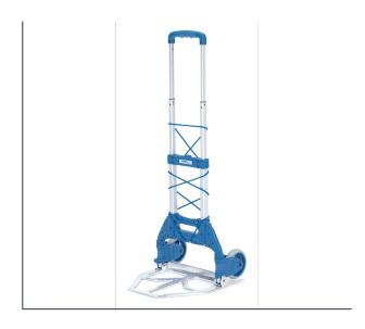
First-class aluminium-steel tube-construction with aluminium blade and premium plastic parts. Non-marking blue-grey polymer wheels, hubs with roller bearings. Hand grip made of comfortable non-slip material. Integral elasticated retaining straps and strip for safe transportation. Blade and wheels foldable with one move, retractable grip. Ready to use within a few seconds.
