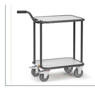
Made of tubular steel welded, handle bolted on. Electrostatic discharge construction, conductive powder coating, slate grey, RAL 7015. 2 electrically conductive wooden shelves according to DIN 68765, light grey. Capacity of upper shelf 100 kg.
