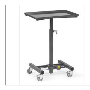
Electrostatic discharge construction. For plastic boxes, steel plate boxes, wire baskets etc., adjustable in height and mobile. Sectional steel-/ tubular construction with steel plate platform with all side rim 20 mm high. Not inclinable. Adjustable in height in intervals of 25 mm. Powder coating, slate grey RAL 7015. 4 swivel castors with TPE-ESD tyres, hubs with slide bearing. Brakes at 2 swivel castors according to the European Standard EN 1757-3 (safety of platform trolleys).
