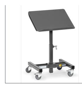
Electrostatic discharge construction. For plastic boxes, steel plate boxes, wire baskets etc., adjustable in height and mobile. Sectional steel-/ tubular construction with steel plate platform with single sided lay-on edge, inclinable by 15° und 30°, adjustable in height in intervals of 25 mm. Powder coating, slate grey RAL 7015. 4 swivel castors with TPE-ESD tyres, hubs with slide bearing. Brakes at 2 swivel castors according to the European Standard EN 1757-3 (safety of platform trolleys).
