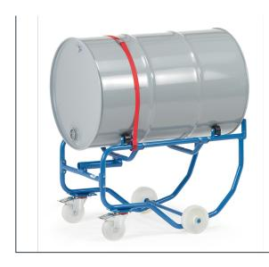
For transporting, storing and draining of 200-litre drums. Tubular steel construction, bolted, powder coated blue RAL 5007. Tension belt to secure the drums. Flat packed for easy self assembly. Fully-fledged mobile drum cradle with lever handle, mobile. With rollers for turning the drums. Applying the drums without lever handle. 2 polyamide castor wheels 125 x 38 mm and 2 polyamide wheels 150 x 40 mm. Castor wheels with wheel lock.
