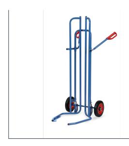
Welded, powder coated, surface durably protected, resistant to impact and scratches. Wheels with solid rubber tyres. Hubs with roller bearings. By activating the hand grips, the truck spreads its carrier spars so that the piles of tyres can be taken up and down directly. Suitable for tyres from 450 up to 750 mm Ø. Up to 8 wheels and tyres possible.
