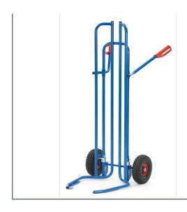
Welded, powder coated, surface durably protected, resistant to impact and scratches. Wheels with pneumatic tyres. Hubs with roller bearings. By activating the hand grips, the truck spreads its carrier spars so that the piles of tyres can be taken up and down directly. Up to 8 wheels and tyres possible.
