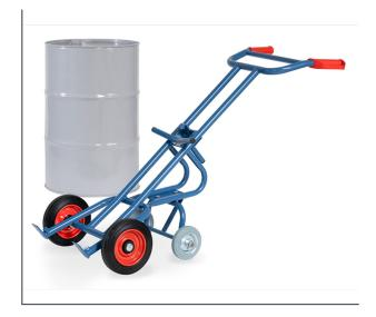
Welded tubular steel, powder-coated, RAL blue 5007, durable surface protection. Wheels with solid rubber tyres, hubs with roller bearings. Suitable for all rimmed 200 litre drums. With 2 additional supporting castor wheels made of solid rubber. With this version, filled barrels can easily be loaded and unloaded from pallets.
