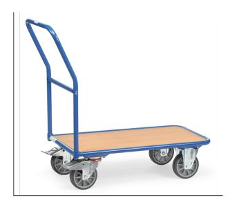
Tubular steel, welded construction, powder coated, blue RAL 5007. Platform made of derived timber material board, beech decor surface. 2 swivel and 2 fixed-wheel castors, TPE tyres, hubs with groove ball bearing. Swivel castors with wheel locks, according to the European Standard EN 1757-3 (safety of platform trolleys).
