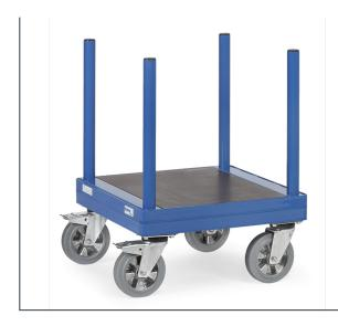
Sectional steel, with insertable tubular steel stanchions, powder coated, blue RAL 5007. Wooden platform proof to water. Heavy duty castor wheels, elasticated solid rubber tyres, blue-grey "trackless" hubs with ball bearings. 2 swivel castors with wheel lock. Clear width between stanchions 510 mm.
