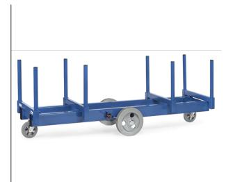
Sectional steel, with insertable tubular steel stanchions, 2 cradles, powder coated, blue RAL 5007. 2 cradles, centre clear for crane or fork-lift loading. Wheels 2113: on centre axle elasticated solid rubber tyres 360 x 75 mm, at each end 1 castor wheel with elasticated solid rubber tyre 200 x 50 mm, blue-grey trackless. Wheel lock on centre axle. Wheels 2123: with Polyurethanee wheels.
