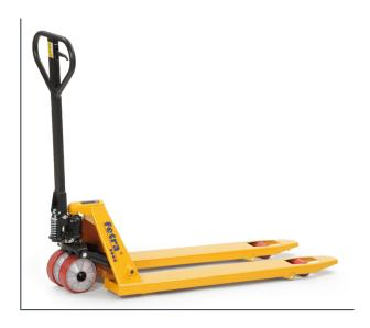
Frames and forks of steel construction, finished powder coated distinct Yellow. Hand hydraulic pump with servicefree bearing. Low maintenance. Strong steel handle powder coated black with counter bearing for pushing operation. Operating lever for lifting, moving, lowering. Steering lock 2 x 100°. Locating wheels at fork tips. Low rolling resistance, non-marking.
