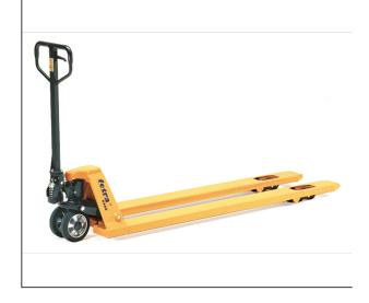
Frames and forks of steel construction, finished powder coated distinct Yellow. Hand hydraulic pump with servicefree bearing. Low maintenance. Strong steel handle with counter bearing for pushing operation. Powder coated black operating lever for lifting, moving, lowering. Steering lock 2 x 100. Locating wheels at fork tips.
