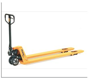
Frames and forks of steel construction, finished powder coated distinct Yellow. Hand hydraulic pump with servicefree bearing. Low maintenance. Strong steel handle with counter bearing for pushing operation. Powder coated black operating lever for lifting, moving, lowering. Steering lock 2 x 100. Locating wheels at fork tips.
