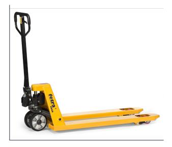
Frames and forks of steel construction, finished powder coated distinct Yellow. Hand hydraulic pump with servicefree bearing. Low maintenance. Strong steel handle with counter bearing for pushing operation. Powder coated black operating lever for lifting, moving, lowering. Steering lock 2 x 100. Locating wheels at fork tips.
