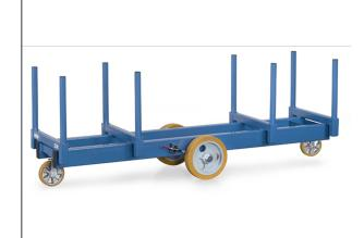
Sectional steel, with insertable tubular steel stanchions, 2 cradles, powder coated, blue RAL 5007. 2 cradles, centre clear for crane or fork-lift loading. Wheels 2113: on centre axle elasticated solid rubber tyres 360 x 75 mm, at each end 1 castor wheel with elasticated solid rubber tyre 200 x 50 mm, blue-grey trackless. Wheel lock on centre axle. Wheels 2123: with Polyurethanee wheels.
