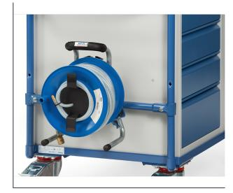
Drum for compressed air hose as a mounting kit for MultiVario table top carts 600 mm wide. Powder-coated blue RAL 5007. Easy assembly to the support tubes of the carts with clamps. 20 m hose, type NW 9. Lockable with padlock (not included in delivery). For models 2401, 2401B, 2401W, 2496, 2496B, 2496W, 2421, 2501, 2501B, 2561, 8101, 8201, 8301, 8241, 8341, 8121, 8221, 8321
