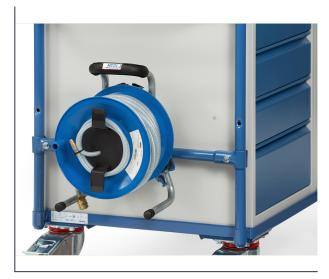
Drum for compressed air hose as a mounting kit for light table top carts 500 mm wide. Powder-coated blue RAL 5007. Easy assembly to the support tubes of the carts with clamps. 20 m hose, type NW 9. Lockable with padlock (not included in delivery). For models 1600, 1800, 2740, 2750, 2940, 2950, 3740, 3760, 4820, 4830, 4920, 4930, 4840
