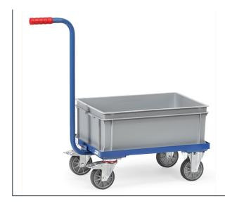
Frame made of angular steel. Shaft with bolt connection, powder coated blue RAL 5007. Frame made of angular steel, with 1 plastic box 600 x 400 x 220 mm, without wooden platform. 2 swivel castors and 2 fixed-wheel castors. Wheels with TPE tyres, hubs with precision deep grove ball bearing. Swivel castors with wheel locks, according to the European Standard EN 1757-3 (safety of platform trolleys).
