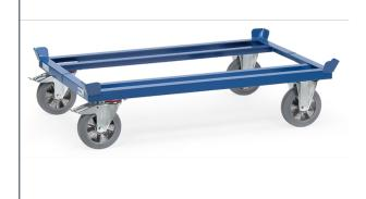
For pallets and boxes. Sturdy sectional steel construction with 4 catch corners for stacking, powder coated. 2 castor wheels and 2 fixed wheels 200 x 50 mm. Castors with wheel lock, according to the European Standard EN 1757-3 (safety of platform trolleys). Elasticated solid rubber tyres, blue-grey "trackless", hubs with ball bearings. Low rolling resistance, easy movement, no road noise. Optional extras are only delivered in a set with pallet dollies because they are welded together.
