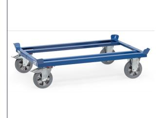
For pallets and boxes. Sturdy sectional steel construction with 4 catch corners for stacking, powder coated. 2 castor wheels and 2 fixed wheels 200 x 50 mm. Castors with wheel lock, according to the European Standard EN 1757-3 (safety of platform trolleys). Elasticated solid rubber tyres, blue-grey "trackless", hubs with ball bearings. Low rolling resistance, easy movement, no road noise. Optional extras are only delivered in a set with pallet dollies because they are welded together.
