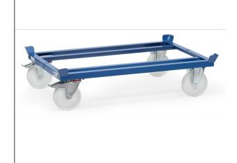
For pallets and boxes. Sturdy sectional steel construction with 4 catch corners for stacking, powder coated. 2 swivel and 2 fixed- wheels 200 x 50 mm. Swivel castors with wheel lock, according to the European Standard EN 1757-3 (safety of platform trolleys). Polyamide wheels, hubs with roller bearings. Low rolling resistance, high chemical resistance, non marking. Road noise. Optional extras are only delivered in a set with pallet dollies because they are welded together.
