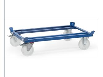
For pallets and boxes. Sturdy sectional steel construction with 4 catch corners for stacking, powder coated. 2 swivel and 2 fixed- wheels 200 x 50 mm. Swivel castors with wheel lock, according to the European Standard EN 1757-3 (safety of platform trolleys). Polyamide wheels, hubs with roller bearings. Low rolling resistance, high chemical resistance, non marking. Road noise. Optional extras are only delivered in a set with pallet dollies because they are welded together.
