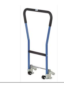
Self-locking push handle for pallet dollies. For comfortable and ergonomic moving of empty and loaded pallet dollies. Sturdy tubular steel construction with strong support claws. Handle and cross tube with softgrip. In unlocked position movable via two auxiliary rollers. Patent pending 10 2014 010 269.9
