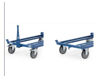
For the transport with towing vehicles up to 6 km/h. Transports up to 5 pallet dollies possible. Maximum train weight 2000 kg. Shaft made of sheet steel. Shaft raises automatically via gas springs into vertical resting position. Robust coupling pin on the fixed-wheel side. Connection via foot operation possible.
