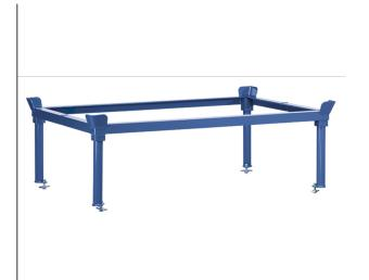
For parking flat pallets and pallet cages at an ergonomically, comfortable level. Angle steel construction with catch corners, sturdy tubular supports with base plates. Stable support tubes with foot plates, to be inserted into corner sleeves at the stacking frame. Powder coated, blue RAL 5007. Stacking frames can be bolted tight with the pallet dolly via base plates and bolting set (included in delivery).
