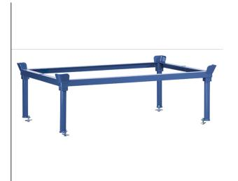
For parking flat pallets and pallet cages at an ergonomically comfortable level. Angle steel construction with catch corners, sturdy tubular supports with base plates. Stable support tubes with foot plates, to be inserted into corner sleeves at the stacking frame. Powder coated, blue RAL 5007. Stacking frames can be bolted tight with the pallet dolly via base plates and bolting set (included in delivery).
