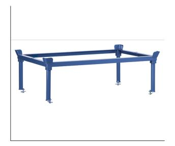
For parking flat pallets and pallet cages at an ergonomically comfortable level. Angle steel construction with catch corners, sturdy tubular supports with base plates. Stable support tubes with foot plates, to be inserted into corner sleeves at the stacking frame. Powder coated, blue RAL 5007. Stacking frames can be bolted tight with the pallet dolly via base plates and bolting set (included in delivery).
