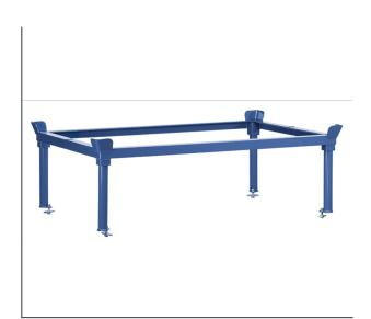
For parking flat pallets and pallet cages at an ergonomically comfortable level. Angle steel construction with catch corners, sturdy tubular supports with base plates. Stable support tubes with foot plates, to be inserted into corner sleeves at the stacking frame. Powder coated, blue RAL 5007. Stacking frames can be bolted tight with the pallet dolly via base plates and bolting set (included in delivery).
