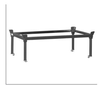
For parking flat pallets and pallet cages at an ergonomically comfortable level. Angle steel construction with catch corners, sturdy tubular supports with base plates. Stable support tubes with foot plates, to be inserted into corner sleeves at the stacking frame. Powder coated, anthracite grey RAL 7016. Stacking frames can be bolted tight with the pallet dolly via base plates and bolting set (included in delivery).
