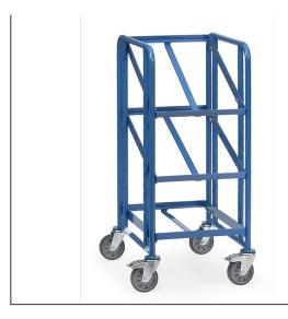
Tubular and sectional steel construction, bolted, powder coated. Open frame. Variable use of shelf frames, distance 50 mm, angle when inclined up to 15° and 30°. 4 swivel castors with TPE tyres, hubs with groove ball bearing. 2 Swivel castors with wheel locks, according to European Standard EN1757-3 (safety of platform trolleys). Capacity upper and middle shelves 80 kg.
