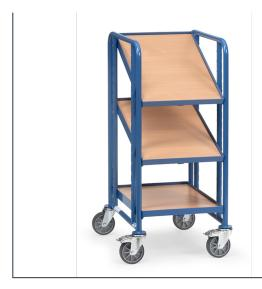
Tubular and sectional steel construction, bolted, powder coated. With 3 platforms with derived timber material boards, rim 10 mm hight. Variable use of shelf frames, distance 50 mm, angle when inclined up to 15° and 30°. 4 swivel castors with TPE tyres, hubs with groove ball bearing. 2 Swivel castors with wheel locks, according to European Standard EN1757-3 (safety of platform trolleys). Capacity upper and middle shelves 80 kg.
