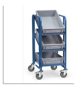
Tubular and sectional steel construction, bolted, powder-coated. Open frames with 3 Euro boxes 600 x 400 x 145 mm . Variable use of shelf frames, distance 50 mm, angle when inclined up to 15° and 30°. 4 swivel castors with TPE tyres, hubs with groove ball bearing. 2 Swivel castors with wheel locks, according to European Standard EN1757-3 (safety of platform trolleys). Capacity upper and middle shelves 80 kg.
