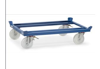
Powder coated in blue RAL 5007. 4 swivel castors with polyamide wheels 200 x 50 mm white, hubs wit precision ball bearings. 2 swivel castors with full locking device in the lead, diagonal layout. Ground clearance: 235 mm
