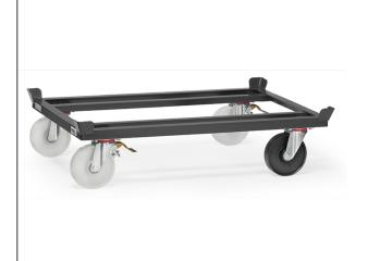
Powder coated in anthracite grey RAL 7016. 3 swivel castors with polyamide wheels 200 x 50 mm white, hubs wit precision ball bearings but 1 castor is electrically conductive, black polypropylene wheel body, hub with precision ball bearings. 2 swivel castors with full locking device in the lead, diagonal layout. Ground clearance: 235 mm
