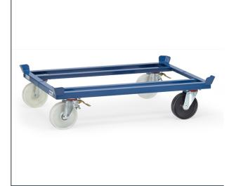
Powder coated in blue RAL 5007. 3 swivel castors with polyamide wheels 200 x 50 mm white, hubs wit precision ball bearings but 1 castor is electrically conductive, black polypropylene wheel body, hub with precision ball bearings.. 2 swivel castors with full locking device in the lead, diagonal layout. Ground clearance: 235 mm
