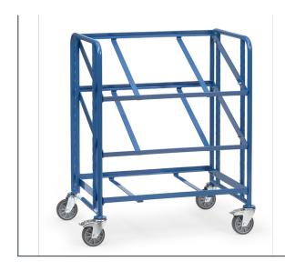
Tubular and sectional steel construction, bolted, powder coated. Open frame. Variable use of shelf frames, distance 50 mm, angle when inclined up to 15° and 30°. 4 swivel castors with TPE tyres, hubs with groove ball bearing. 2 Swivel castors with wheel locks, according to European Standard EN1757-3 (safety of platform trolleys). Capacity upper and middle shelves 80 kg.
