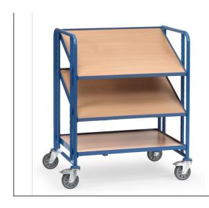
Tubular and sectional steel construction, bolted, powder coated. With 3 platforms with derived timber material boards, rim 10 mm hight. Variable use of shelf frames, distance 50 mm, angle when inclined up to 15° and 30°. 4 swivel castors with TPE tyres, hubs with groove ball bearing. 2 Swivel castors with wheel locks, according to European Standard EN1757-3 (safety of platform trolleys). Capacity upper and middle shelves 80 kg.
