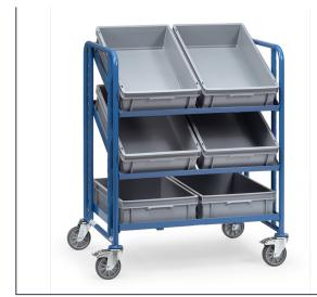
Tubular and sectional steel construction, bolted, powder-coated. Open frames with 6 Euro boxes 600 x 400 x 145 mm . Variable use of shelf frames, distance 50 mm, angle when inclined up to 15° and 30°. 4 swivel castors with TPE tyres, hubs with groove ball bearing. 2 Swivel castors with wheel locks, according to European Standard EN1757-3 (safety of platform trolleys). Capacity upper and middle shelves 80 kg.
