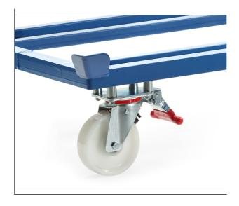
Fixed operating levers underneath the frame, not protruding. To be operated from the long side. Easy reach in any castor position. Ground clearance increased to 237 mm, loading height to 282 mm.
