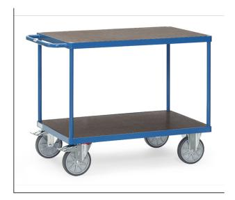
Modular system: Tubular steel and sectional steel, welded and powder coated, surface durably protected, resistant to impact and scratches. 2 shelves with nonslip plywood board. 2 swivel and 2 fixed-wheel castors, TPE tyres, hubs with groove ball bearing. Swivel castors with wheel locks, according to the European Standard EN 1757-3 (safety of platform trolleys). Capacity upper shelf 200 kg.
