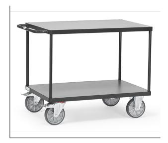
Modular system: Tubular steel and sectional steel, welded and powder coated, surface durably protected, resistant to impact and scratches. 2 shelves made of derived timber material boards, surface grey. 2 swivel and 2 fixed-wheel castors, TPE tyres, hubs with groove ball bearing. Swivel castors with wheel locks, according to the European Standard EN 1757-3 (safety of platform trolleys). Capacity upper shelf 200 kg.
