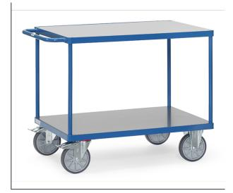
Modular system: Tubular steel and sectional steel, welded and powder coated, surface durably protected, resistant to impact and scratches. 2 shelves with weatherproof rigid PVC panel in dark grey. High chemical resistance, low flammability. 2 swivel and 2 fixed-wheel castors, TPE tyres, hubs with groove ball bearing. Swivel castors with wheel locks, according to the European Standard EN 1757-3 (safety of platform trolleys). Capacity upper shelf 200 kg.
