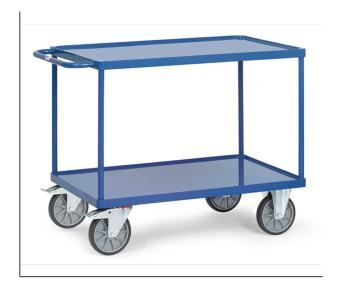
Modular system: Tubular steel and sectional steel, welded and powder coated, surface durably protected, resistant to impact and scratches. 2 platforms, trays made of steel sheet, with rim 10 mm high, welded oil-tight, powder coated. 2 swivel and 2 fixed-wheel castors, TPE tyres, hubs with groove ball bearing. Swivel castors with wheel locks, according to the European Standard EN 1757-3 (safety of platform trolleys). Capacity upper shelf 200 kg.
