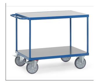
Modular system: Tubular steel and sectional steel, welded and powder coated, surface durably protected, resistant to impact and scratches. 2 shelves with weatherproof rigid PVC panel in dark grey. High chemical resistance, low flammability. 2 swivel and 2 fixed-wheel castors, TPE tyres, hubs with groove ball bearing. Swivel castors with wheel locks, according to the European Standard EN 1757-3 (safety of platform trolleys). Capacity upper shelf 200 kg.
