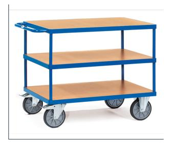
Modular system: Tubular steel and sectional steel, welded and powder coated, surface durably protected, resistant to impact and scratches. 3 shelves made of derived timber material boards, surface beech grain. 2 swivel and 2 fixed-wheel castors, TPE tyres, hubs with groove ball bearing. Swivel castors with wheel locks, according to the European Standard EN 1757-3 (safety of platform trolleys). Capacity upper and middle shelf 200 kg.
