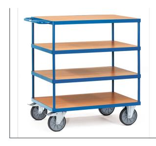
Modular system: Tubular steel and sectional steel, welded and powder coated, surface durably protected, resistant to impact and scratches. 3 shelves made of derived timber material boards, surface beech grain. 2 swivel and 2 fixed-wheel castors, TPE tyres, hubs with groove ball bearing. Swivel castors with wheel locks, according to the European Standard EN 1757-3 (safety of platform trolleys). Capacity upper and middle shelf 200 kg.
