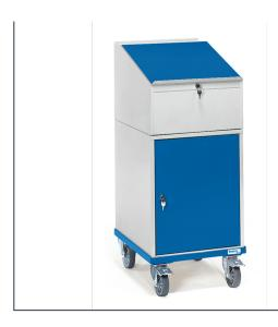
Leaf-door cupboard, lockable, 1 fixed and 2 adjustable shelves, 500 mm wide, 600 mm deep and 600 mm high. Fit-on desk-top made of powder-coated steel plate. Desktop foldable. 4 swivel castors with TPE tyres, hubs with groove ball bearing. 2 swivel castors with wheel locks. Powder coated, carcass grey RAL 7035, front blue RAL 5007. Height of surface: 1034,1197 mm, total length: 650 mm, total width: 550 mm. Capacity per shelf 30 kg.
