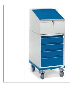
Cupboard of drawers, centrally lockable, 3 drawers 120 mm high and 1 drawer 180 mm high. Ball pull-out and pull-out lock. Fit-on desk-top made of powder-coated steel plate. Desktop foldable. 4 swivel castors with TPE tyres, hubs with groove ball bearing. 2 swivel castors with wheel locks. Powder coated, carcass grey RAL 7035, front blue RAL 5007. Height of surface: 1034/1197 mm, total length: 650 mm, total width: 550 mm. Capacity per drawer 25 kg.
