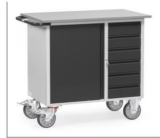
Made of steel sheets with 1 cupboard, 1 fixed and 2 adjustable shelves, and 6 drawers (H x W x D: 95 x 280 x 470 mm) with sliding guide. Centrally lockable by cylinder lock. Powder coated, carcass grey RAL 7035, front anthracite grey RAL 7016. Worktop composite panel grey 20 mm. 2 swivel and 2 fixed-wheel castors, TPE tyres, hubs with groove ball bearing. Swivel castors with wheel locks, according to the European Standard EN 1757-3 (safety of platform trolleys).
